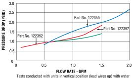
Tests conducted with units in vertical position (lead wires up) with water at +70 F (21 C).
