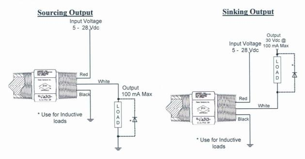
Note: Must maintain suitable ground through metallic housing or equipment interconnection.
